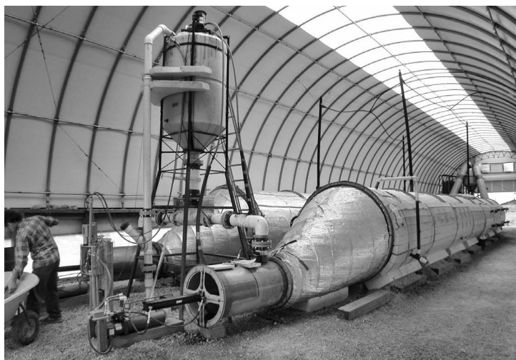
Avatar 80 cow pilot system built with two 6' diameter hulls.
